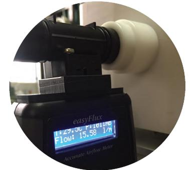
Adjust the flow rate up to reach the desired value in the display of easyFlux. in easySPT100 by using the button - and + on the rear user interface. In the easySPT200 by using a screw driver to rotate the flow rate screw under the nozzle.
